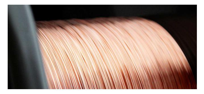
This is copper wire for micro-catheters developed to focus on releasability from resin and reduction of wire surface contamination.
